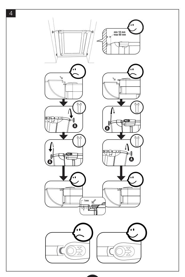
To open the gate, slide the latch away from the wall (1) and lift the gate (2). The gate should open both ways. The arrows on the top of the latch indicate the direction in which the gate can be opened. Two green arrows indicate that the gate can be opened in either direction
