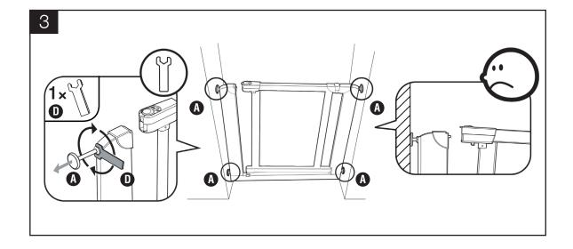
The distance between the wall surface and the gate should be no less than 18mm and no more than 60mm on both sides.
